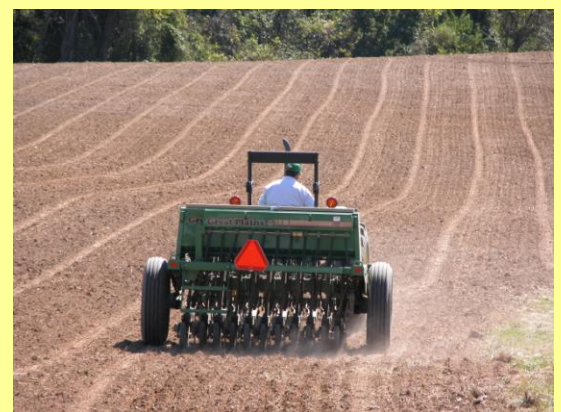
Sowing Cover Crops with SCD's Great Plains 7 foot No Till Planter
